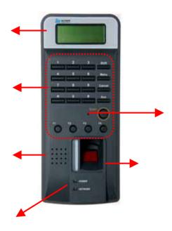
LCD: All activities are displayed with text message. Key pad: Used for ID input and environment setting. Details are as follows.
